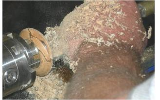
Having done the front face, it's sanded and treated, then reversed in the chuck and the back of the watch completed. The fob on the top was made from a small piece of ebony, which was not demonstrated. The ring at the top is from a key ring.
